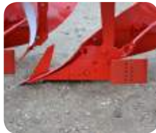
Landslide wear plate.
