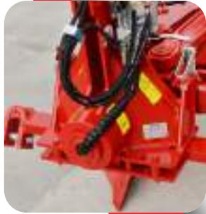
Hollow shaft allowing optimal hose passage.
