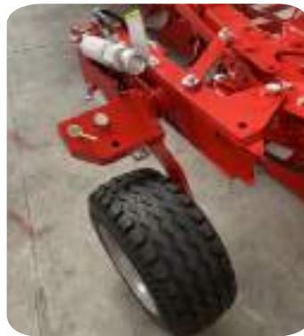
Advanced hydraulic transport and control wheel 340/55 16"
