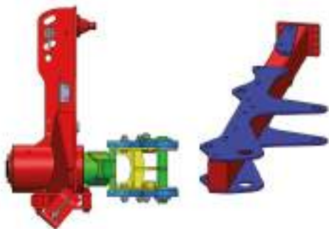
Headstock 130 + frame support 130 + 150*100 mm frame section.
