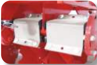
Auto reset protection by means of rubber suspensions with special anti-slip shape.
