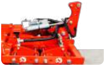
Hydraulic frame lift to decrease weight on the tractor lower arms.
