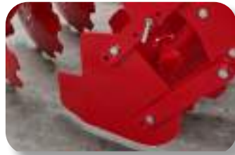
Side plates with parallelogram linkage.
