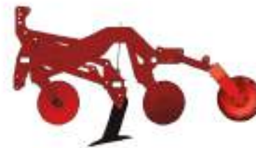
The 600 mm tines can operate up to 25 cm below the working depth of the discs.
