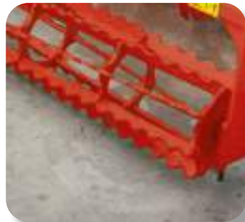
400 mm or 520 mm notched plate roller.
