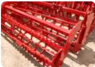
480 mm bar tandem roller + 400 mm notched roller (150 kg/m)
