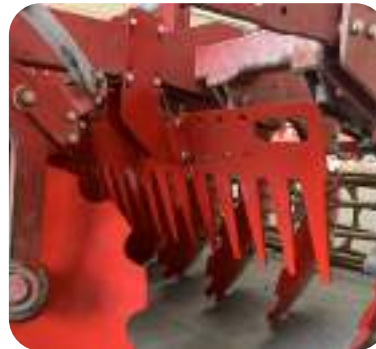
Tined rake placed between the disc rows or between discs and the roller to stop the flow of earth and tear it to pieces. (Optional).
