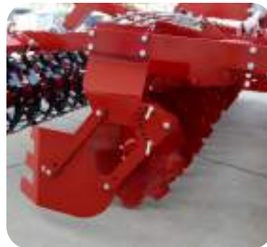
Side deflectors with parallelogram (Optional)
