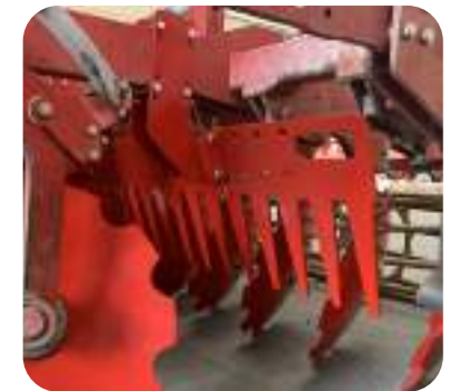
Tined rake placed between the rows of discs or between the discs and the roller to slow down the flow of soil and break it up (Optional).
