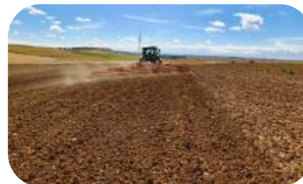
Perfect finish, typical of a seedbed cultivator, thanks to the levelling boards and the rear roller.
