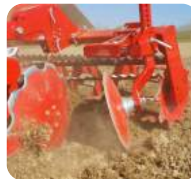
Limiting left side disc to close the furrow made by the rear left disc. (Optional).
