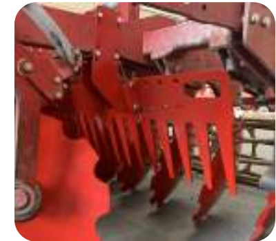
Tined rake placed between the disc rows or between discs and the roller to stop the flow of earth and tear it to pieces. (Optional).
