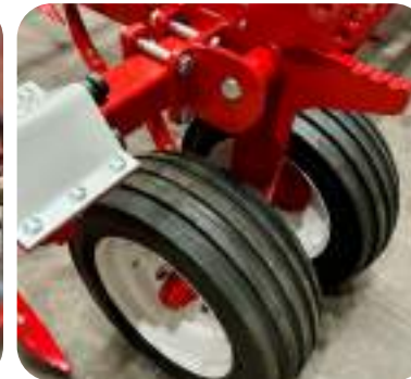
Double front wheels 200/60 14.5' with hydraulic folding for transport (standard).
