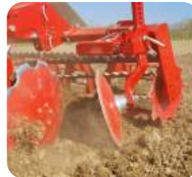
Left edge disc to close the furrow formed by the left rear disc. (Optional).
