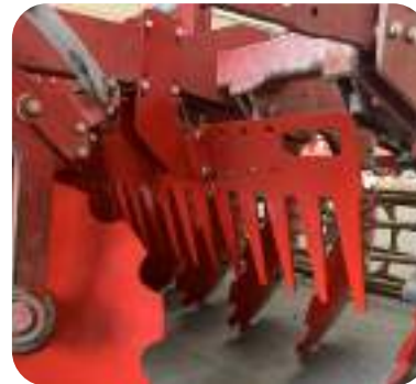
Tined rake placed between the disc rows or between discs and the roller to stop the flow of earth and tear it to pieces. (Optional).
