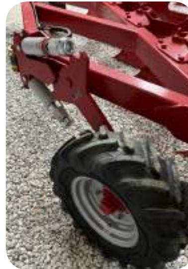
Hydraulic depth control or combi wheel for transport and depth control
