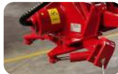
Oscillating shaft with shock absorption
