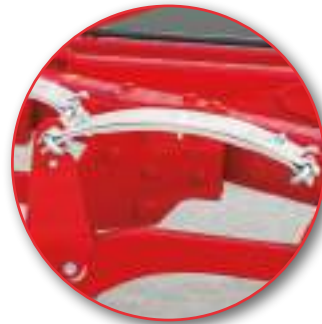
Leafspring security system: Mini-BF
