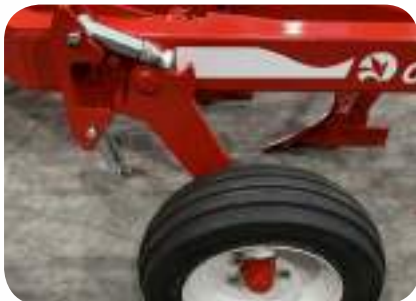
Depth control wheel. Available as 6.00*9", 200/60, 250/65, 340/55, 280/70 y 380/55
