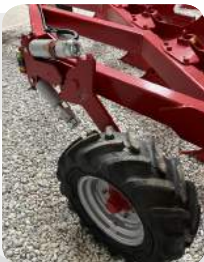
Hydraulic depth control or combi wheel for transport and depth control
