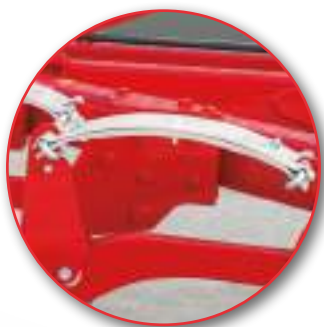
Leafspring security system: Mini-BF
