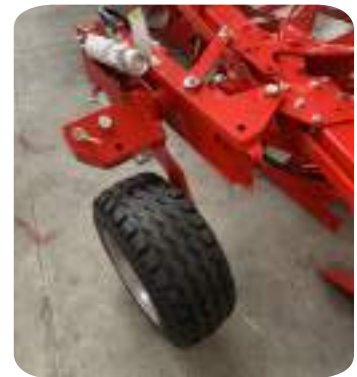
Advanced hydraulic transport and control wheel 340/55 16"
