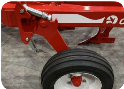
Depth control wheel. Available as 6.00*9, 200/60, 250/65, 340/55, 280/70 y 380/55
