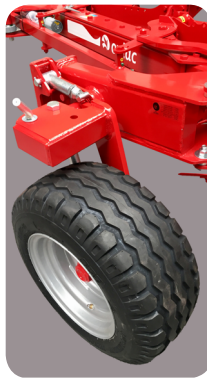
Advanced depth and transport wheel 340.
