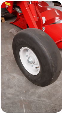
Rear depth control wheel 550/65.
