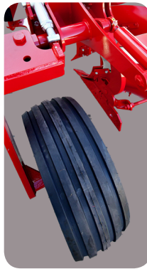
Rear depth and transport wheel 250.
