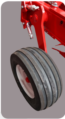
Advanced depth control wheel 250.
