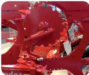
Smooth or Notched Coulter Discs with Non Stop Security System.
