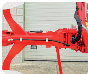
X-Light beam, 25 kg lighter than standard one (Max: 32 HP per body). Available solely for 130 series.
