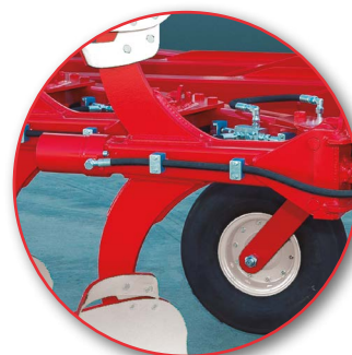
Hydraulic release system. Mini-HF, Mini-NH and Mini-SH
