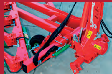
Hydraulic first furrow adjustment
