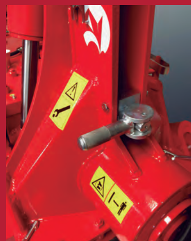
Headstock lock for transport
