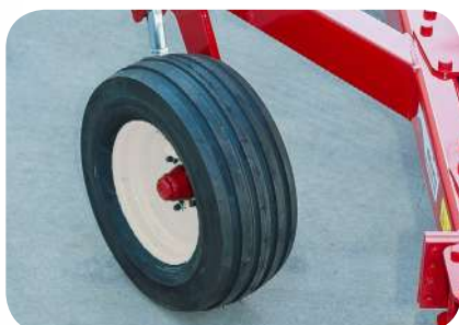
Rear depth control wheel. Available as 6.00*9", 200/60 14,5", 250/65 14,5", 340/55 16" and 380/55 17"
