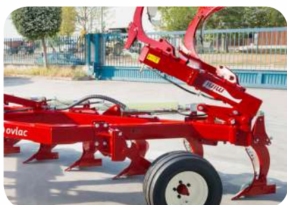
Hydraulically foldable rear bodies (for Mini BF and HF)
