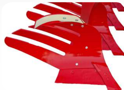
Slatted mouldboards for sticky conditions- Trashboards to improve burial of trash
