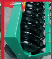
The side plates and end discs limit land projections outwardly to finish perfectly level.
