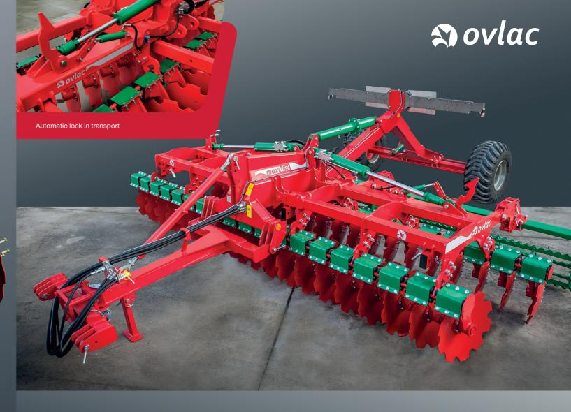
Any mounted *Maxidisc II* can be transformed into trailed by just mounting the **Trail Kit.**The draw bar is mounted right on the three point linkage of the *Maxidisc II* and it offers a category II/III linkage on the lifting arms of the tractor. Its height can be easily adjusted by means of the turnbuckle on the third point. The wheel chassis is also mounted directly at the rear of the main frame and features hydraulic suspension as well as hydraulic or
