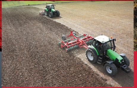
Short disc harrows have become over the last years one of the fastest and more efficient ways of tillage. An intense action of chopping and mixing results in a very effective way to incorporate trash and to make weeds germinate for an ulterior final treatment.
