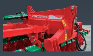
The *Maxidisc II* offers a solid structure calculated to stand the high forces derived from the use of 24" discs as well as big tractors. Category II and III linkage.
